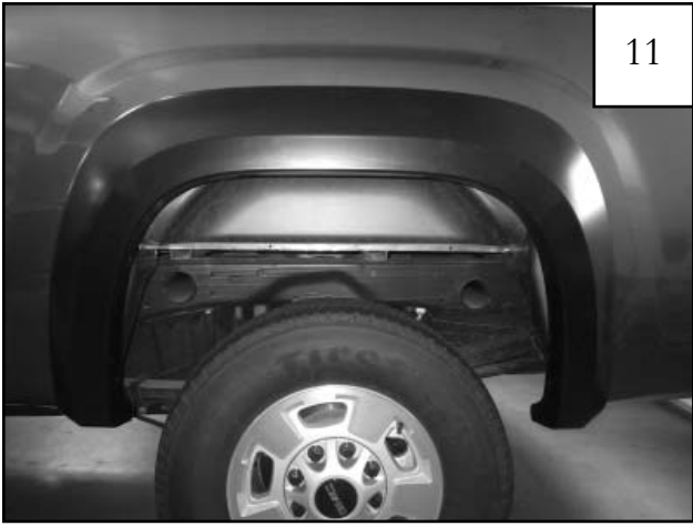
Completed rear flare installation.
